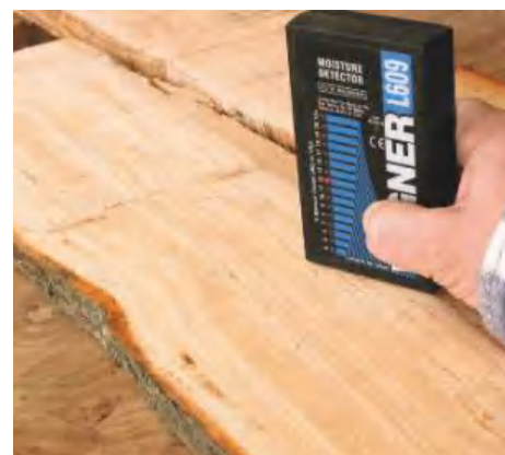
▲ Pic.8 A moisture meter reads the percentage of water left in the wood
